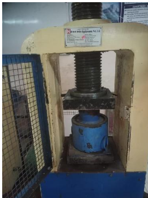
Figure 5.12: Crushing Test on Plastic Aggregate.
