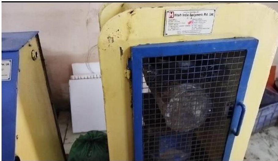
Figure 5.19: Teston Flexural Strength in CTM
