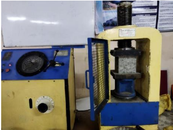
Figure 5.17: Concrete Cube Tested on CTM
